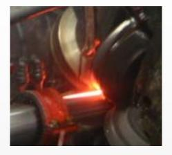
Two color eye indicates precise temperature only if a part of the object to be measured stays in a part of the scope of viewing area of the glass fiber eye.
