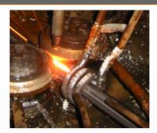
In case of the controller is not used. (Welding temperature fluctuates due to hoop thickness and line speed.)
